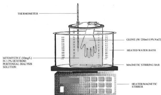
FIG. 1. Apparatus for testing the mitomycin C penetration of latex sterile gloves.
